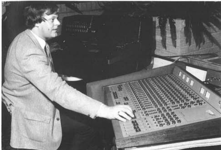
Granada Theatres' stage manager Ian Sopp pictured at the controls in 1983. The sound control in the foreground is System 8, and the lighting control in the background an extended Pulsar outfit that was a mixture of rock desks, matrix extenders and modulators, etc. This was later replaced by a Celco Series 2 30 way board.
