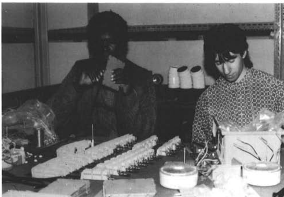
A special job: assembly of transformers for Light Plan Consultants - part of a projects for a Dulux concession presentation for Texas Homecare at Dudley in the West Midlands.
